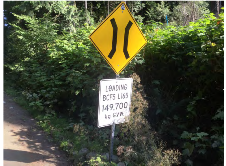
Load Rating Sign
